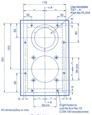
The B110A is mounted behind the baffle. Therefore the back panel must be removable.
