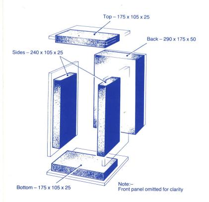
Pads of sound absorbing material are placed inside the cabinet to inhibit the formation of standing waves in the enclosed air space. Suitable materials include polyester foam, resin-bonded fibre glass and acetate fibre. The pads are retained by adhesive or string lacing.
